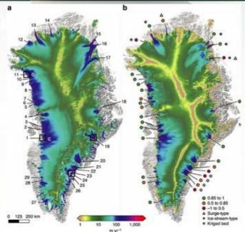
Left: Surface speeds for Greenland for 2008-2009. a. Observed speeds. adjusted to represent annual averages; b. Calibrated model speeds at 600-m grid resolution.
